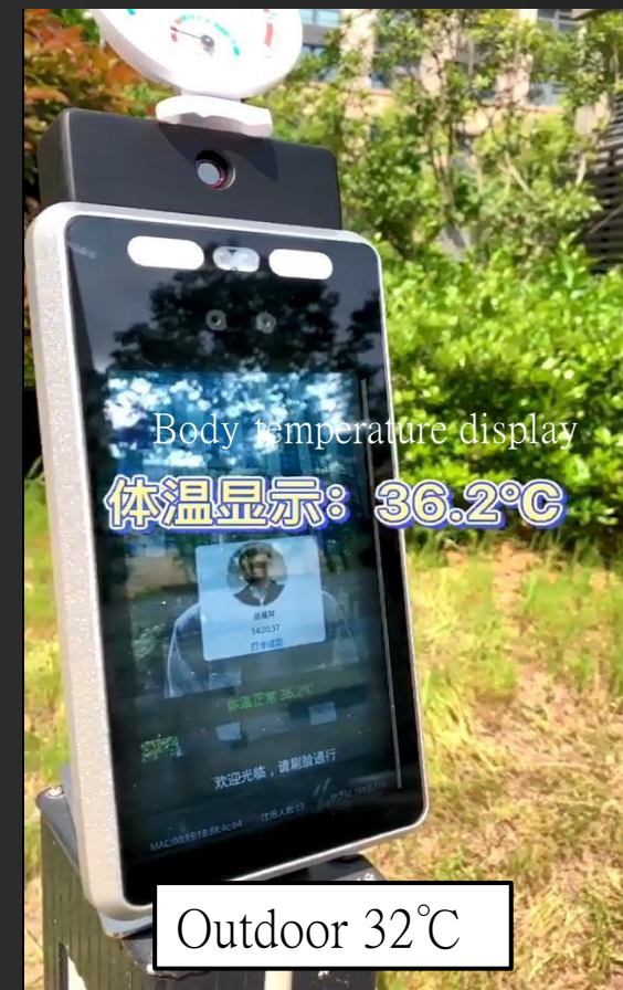
DJS-F10 still maintains <math><0.3</math> temperature measurement accuracy in different environments
