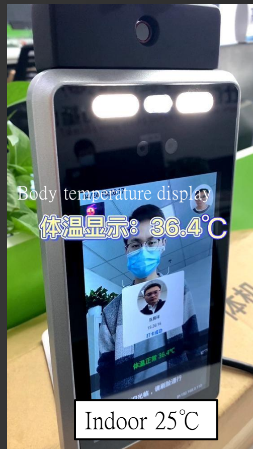
DJS-F10 still maintains <math><0.3</math> temperature measurement accuracy in different environments
